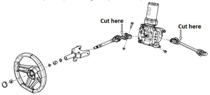
2018-24 Can-Am DPS has an additional bracket welded over the 2017 location. You will need to use a cut off wheel and grinder to remove this bracket (marked in red on the below left diagram). You will then drill out the 4 holes (marked in red on below right diagram) to mount the ePowerSteering bracket. Also note that the steering assembly mount has enlarged holes. You may need to loosen and reposition it.
