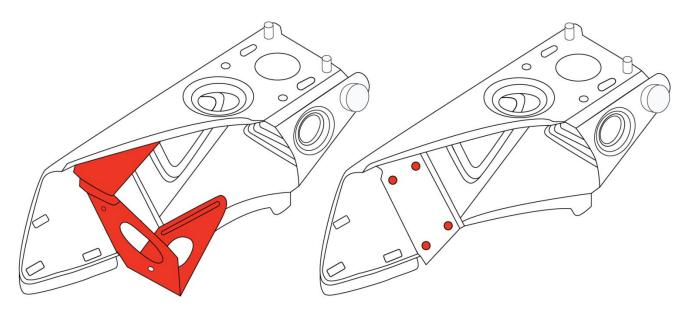
Use the X3's 1.25" tube to the left of the steering wheel to mount the ECU bracket to the frame. This will
