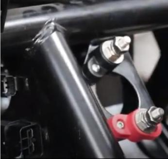
Install the ECU mount onto the center of the horizontal chassis tube under the most forward part of the dash using the included hose clamps. See below.
